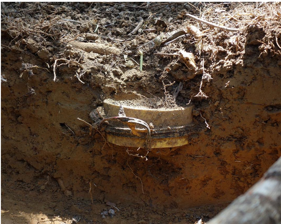
Typical AP mine laying: a 'betun' type AP mine found buried 3cm below the surface in Colombia. Photo courtesy of E. Chrystie
