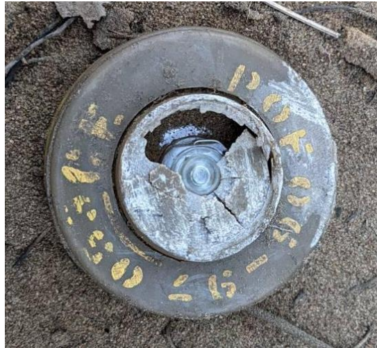
A degraded P4 anti-personnel mine. As the casing degrades over time, the explosive fill (tetryl) can leach out. Photo courtesy of E. Chrystie
