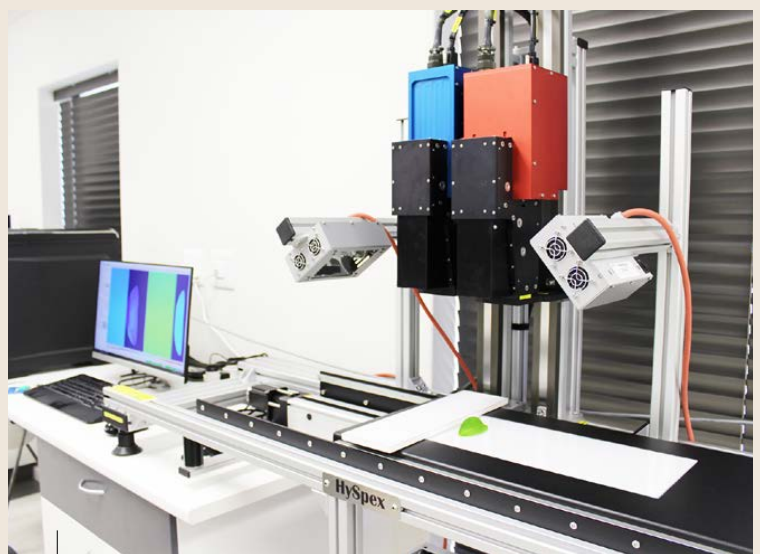
SU’s hyperspectral imaging system can be used to acquire spectra of samples in the visible near-infrared and shortwave infrared wavelengths. Photo supplied
